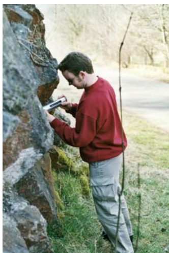
Fig 5.1 Using a Schmidt hammer at Apes Tor
